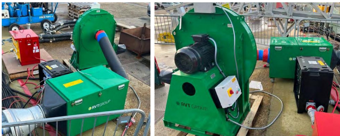
VENTEX ® Centrifugal Fan 200S-HP working in conjunction with RVT's RAVEX ® Wandafilta Plus Fume Extraction & Filtration Kit
