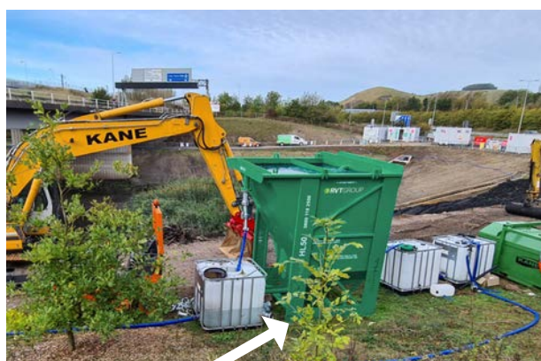
The HL50 is RVT's largest settlement tank, designed to remove suspended solid particles from water (50m 2 volume)
