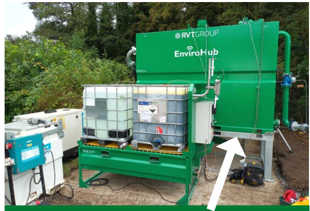
Treatment Tanks are designed to pre-treat water with coagulant and flocculent polymer to improve settlement of solids, or for pH correction
