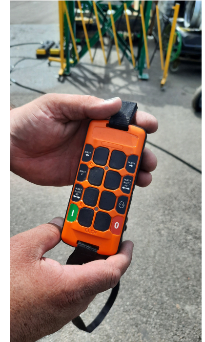
Pictured above is the remote control which enables you to switch the unit on/off and control oscillation of the jet."
