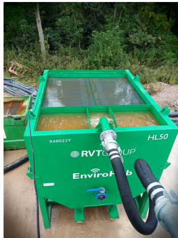
Lamella Plate Settlement Tank removing suspended solid particles from water (50m 3 volume).
