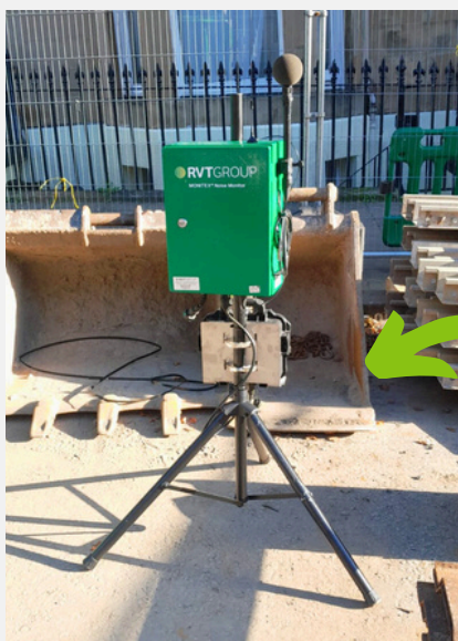
MONITEX® Environmental Noise Monitor in use on the project.
