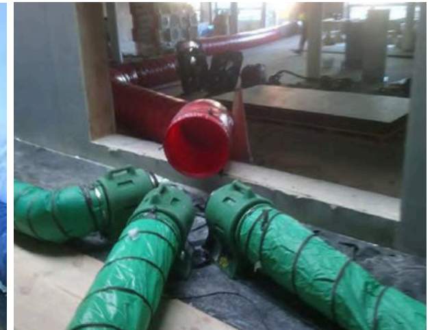
The indirect oil fired heater forces warm air along the ducting, into the sealed building, where it can be evenly distributed using air distribution kits.
