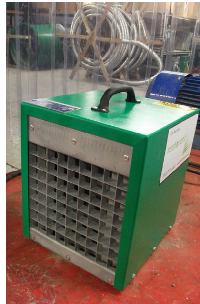
Example of electric heater used to dry out paint work and provide ambient heat whilst other trades continue working.
