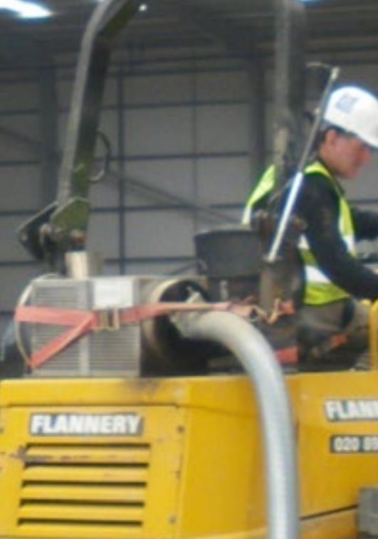
Image above of a diesel particulate filter.
